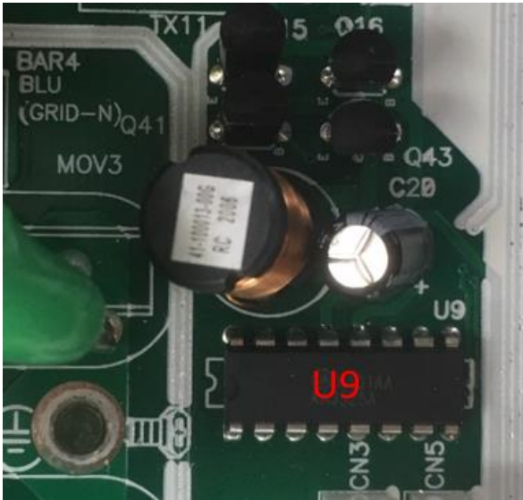
The U9 is (IC PWM CNTL ON/KA3525A)
