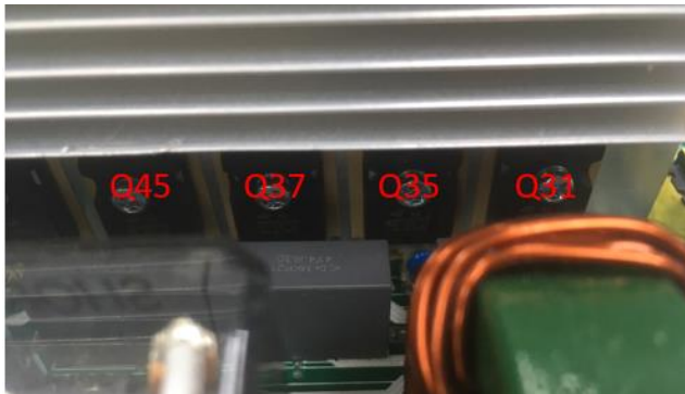
For AXPERT MAX II 8KW ALL of the IGBTs are (IGBT ST/STGW60H65DFB 60A 650V N BULK TO-247)
